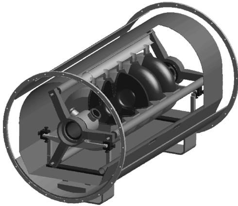
Figure 5: Preliminary design for the 4.2 K cryostat.
