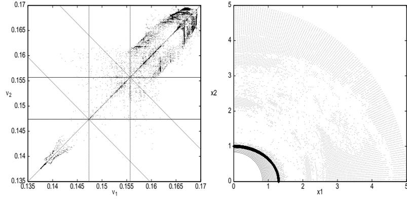
FIGURE 5: F.M. for the case #1, with 30% beam mismatch ( $\delta_1 = 0.3, \delta_2 = 0$ ). On the left side resonance lines with  $|k_1| + |k_2| + |h_-| + |h_+| \leq 3$  are plotted. The initial beam envelope is drawn on right side, together with regular points.
