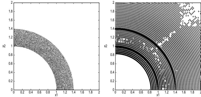
FIGURE 8: Results of tracking for case #1, matched. On the left point 10 000 initial conditions chosen for tracking are shown; different markers are used for the point that diffuse up to  $r_{\max} \geq 2$  (no one in this case). In the left plot for comparison the result of the F.M. analysis on the same scale is shown; The annulus used for tracking initial conditions is also drawn.
