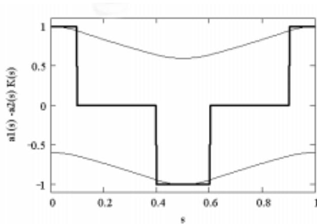
FIGURE 1: Geometry of the nominal FODO cell 1m long; the focusing function  $K(s) = K_1(s) = -K_2(s)$  is plotted, together with the matched envelopes  $a_1$  and  $-a_2$  in arbitrary units.
