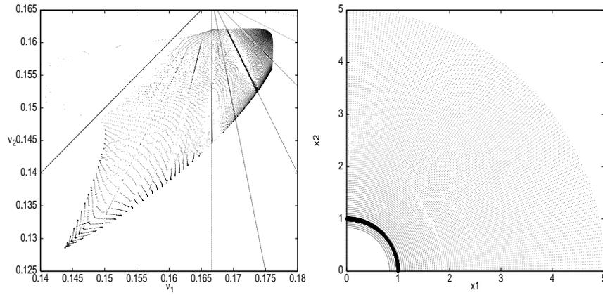
FIGURE 6: F.M. for the case #2, matched beam; in the left plot resonance lines with  $|k_1| + |k_2| \leq 6$  are plotted. In the right plot regular points and beam cross section are shown.
