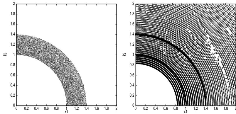
FIGURE 10: Results of tracking for case #2, matched. On the left point 10 000 initial conditions chosen for tracking are shown; different markers are used for the point that diffuse up to  $r_{\max} \geq 2$ (no one in this case). In the right plot for comparison the result of the F.M. analysis on the same scale is shown.
