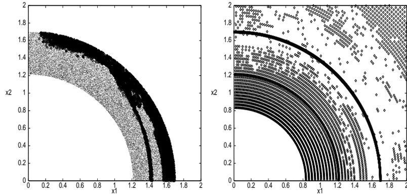
FIGURE 11: Results of tracking for case #2, mismatched ( $\delta_1 = \delta_2 = .3/\sqrt{2}$ ). On the left point 10 000 initial conditions chosen for tracking are shown; different markers are used for the point that diffuse up to  $r_{\max} \geq 2$ . In the right plot for comparison the result of the F.M. analysis on the same scale is shown.
