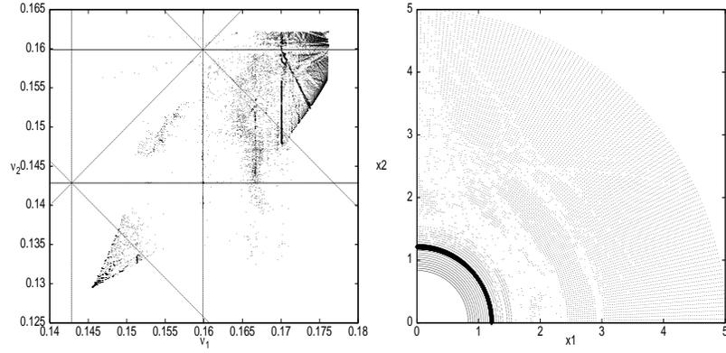
FIGURE 7: F.M. for the case #2,  $\delta_1 = 0.3/\sqrt{2}$ ,  $\delta_2 = 0.3/\sqrt{2}$ . On the left side resonance lines with  $|k_1| + |k_2| + |h_-| + |h_+| \leq 3$  are plotted. The initial beam envelope is drawn on right side, together with regular points.
