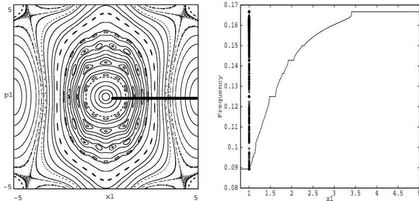
FIGURE 2: One degree of freedom Poincaré Map and Frequency Map for a matched beam propagating in our nominal FODO ( $\xi = 3 * 10^{-6}$ ,  $K_F = K_D = 12$ ,  $x_2 = p_2 = 0$ ).
