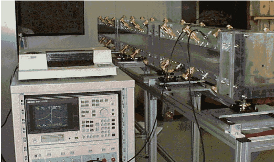
Figure 1. The Aluminum model of the RFQ prototype under RF test at LNL.
