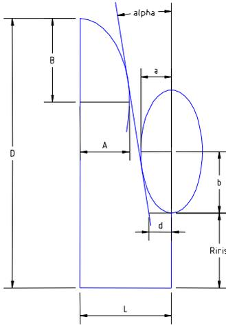
Figure 2: Reference geometry for the cavity shape.
