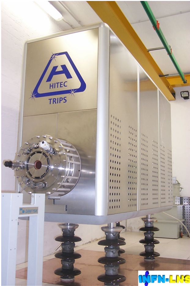
Figure 7: The 100 kV high voltage platform.
