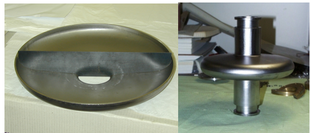
Figure 1. A 700 MHz \beta=0.5 niobium half-cell deep drawn by Zanon, ready for welding, and a scaled (one half) single cell cavity.
