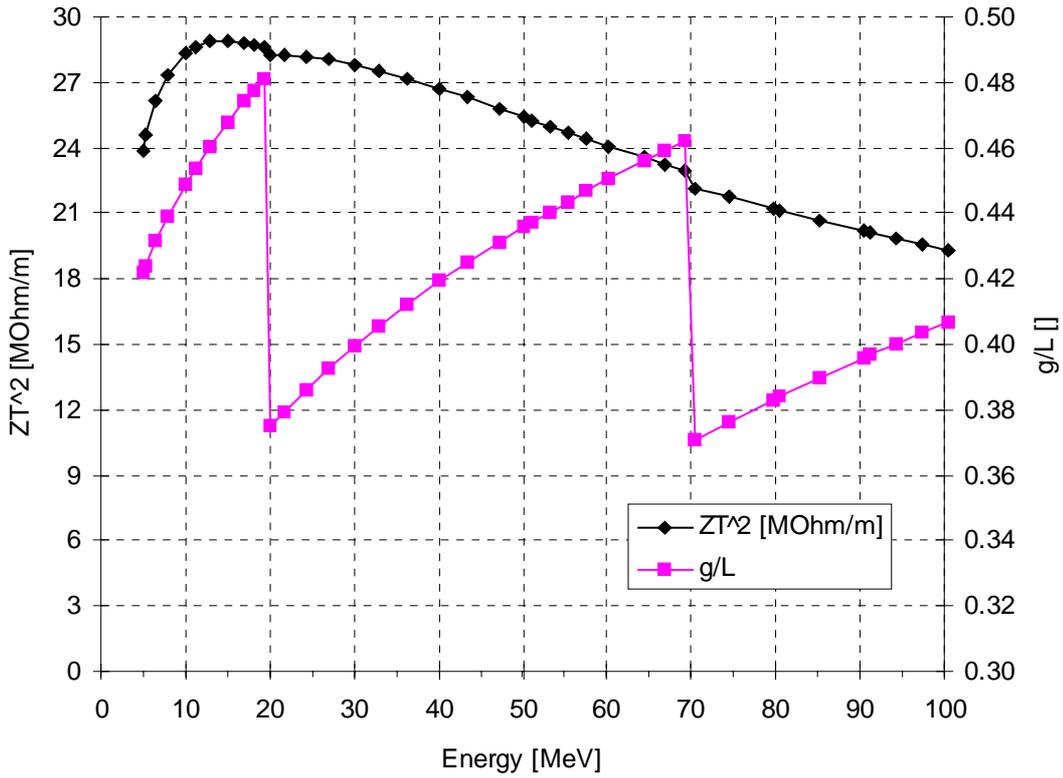
Figure 5: Effective shunt impedance and gap over cell length ratio as function of energy in the DTL.
