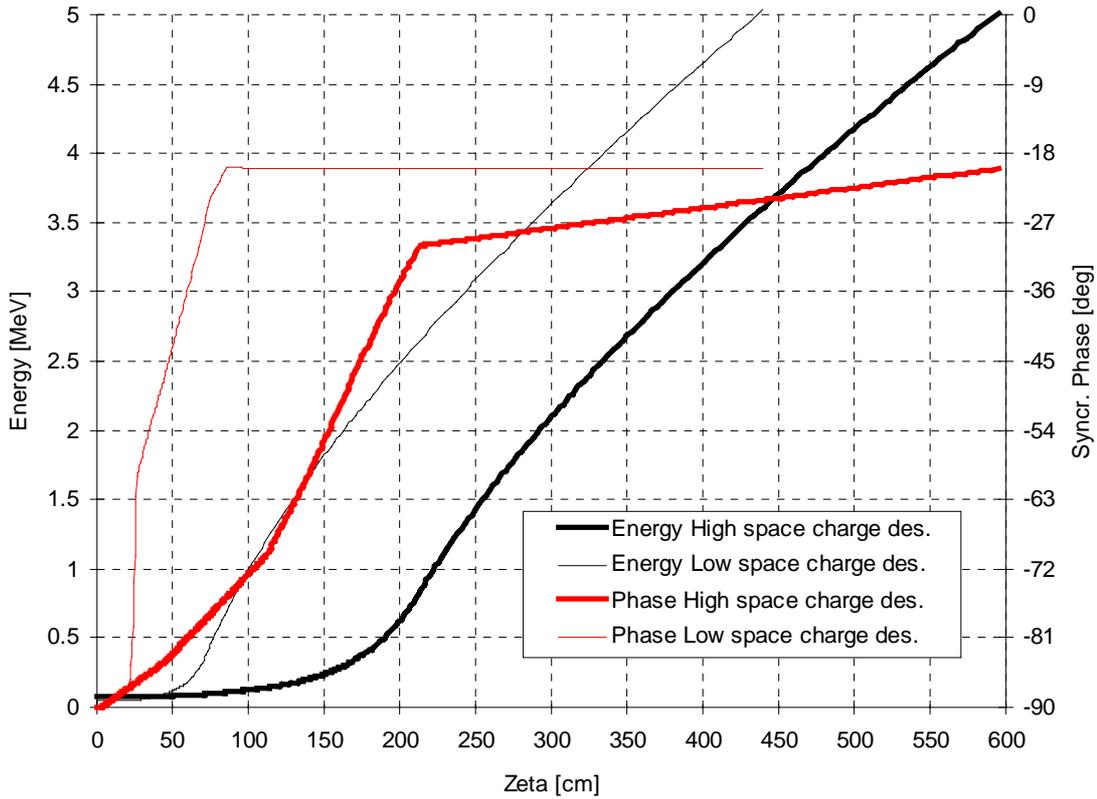
Figure 2: Synchronous particle energy and phase in the RFQ as a function of length; high space charge and low space charge design technique are used
