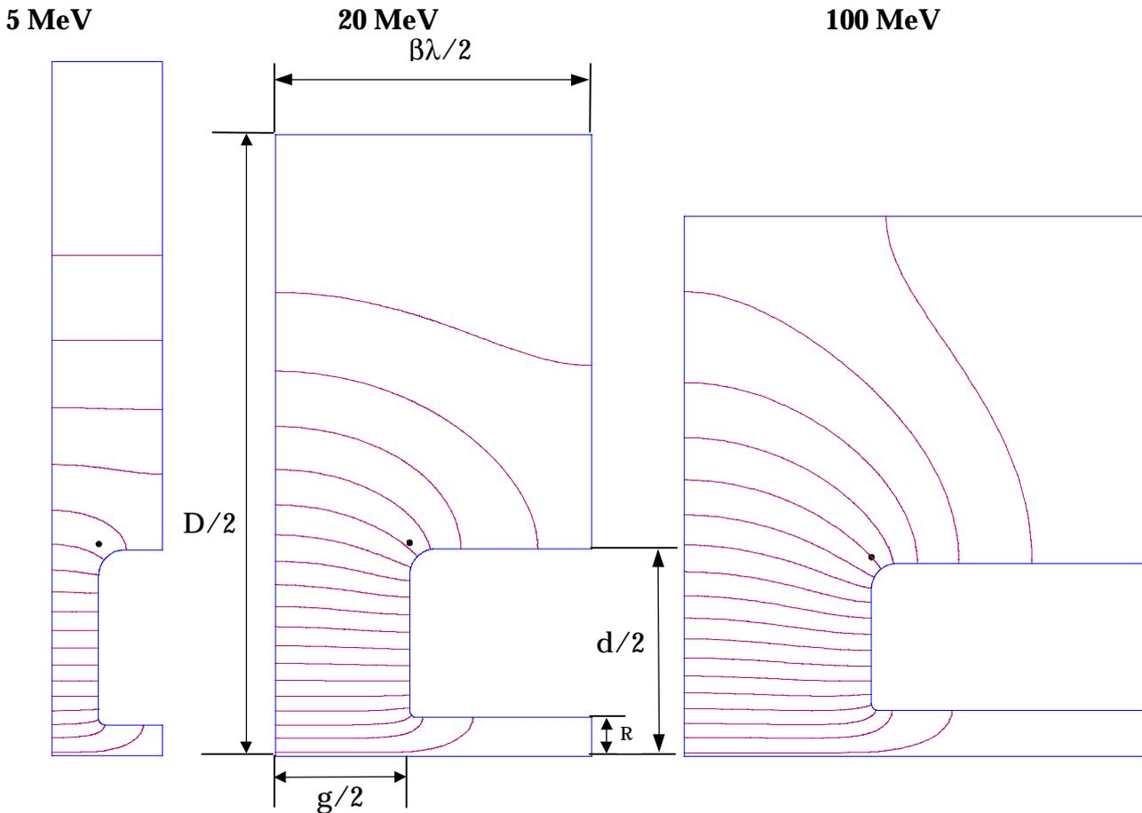
Figure 6: Cell geometry and electric field for different energies in the DTL.
