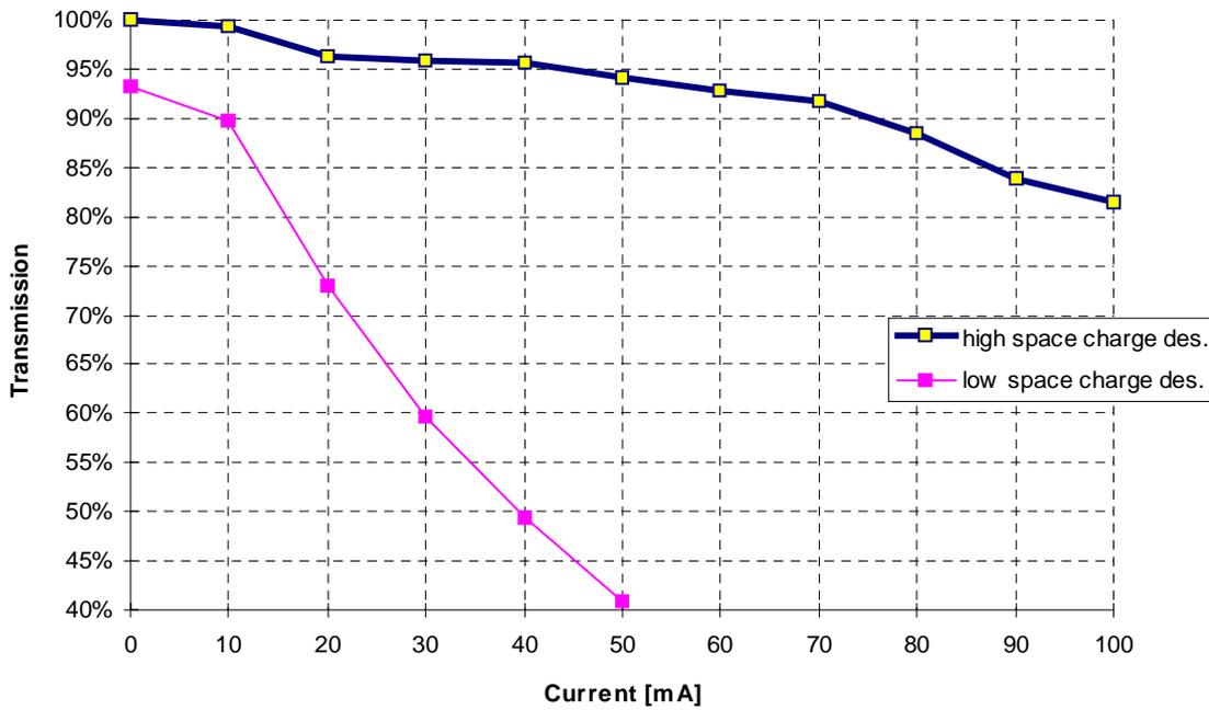
Figure 3: RFQ transmission as a function of beam current for low space charge and high space charge design.
