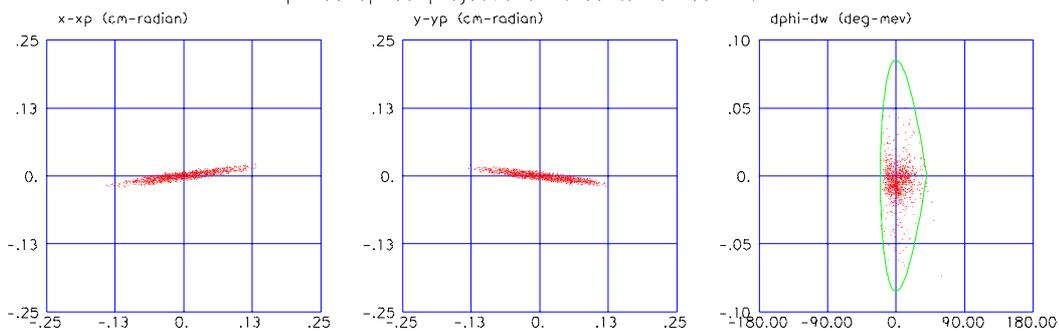
Figure 4: Beam profiles, initial and final phase space in the RFQ (30 mA beam current)
