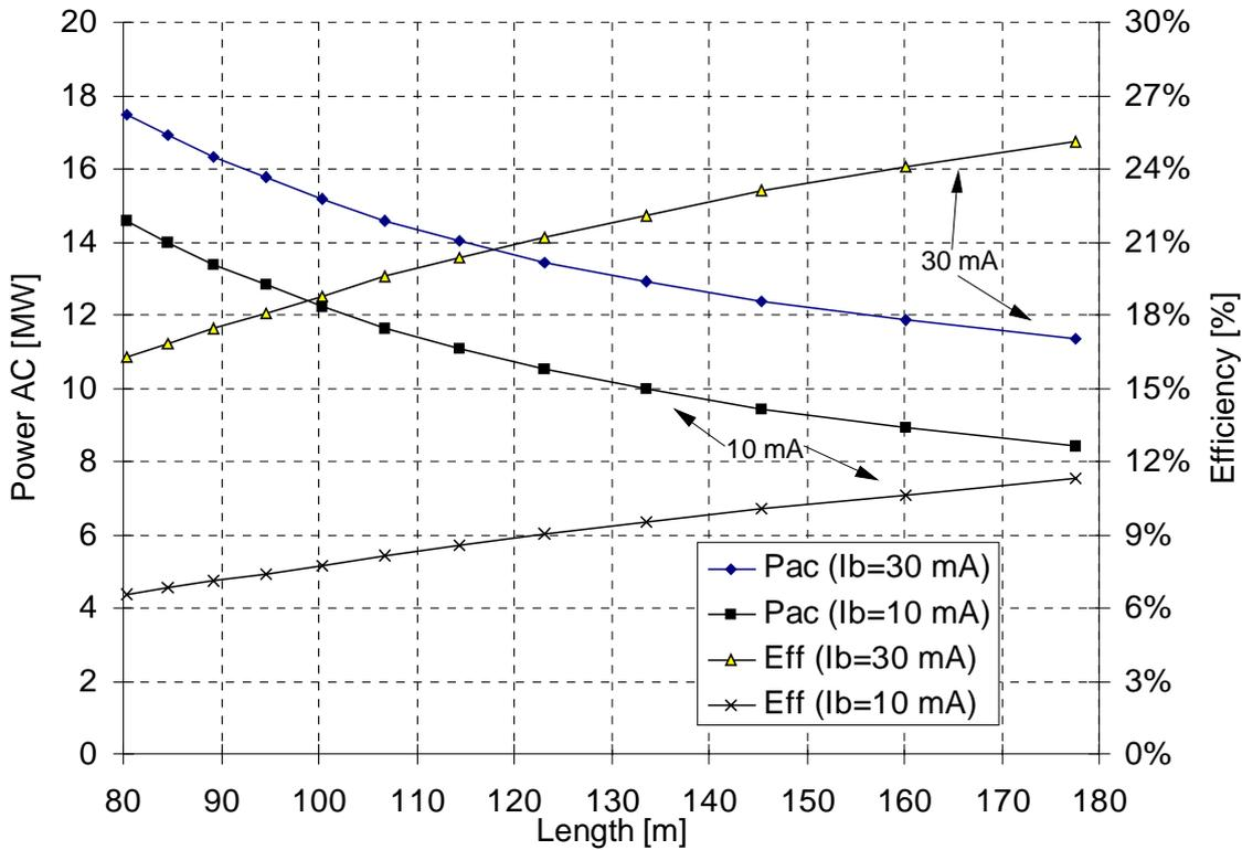
Figure 8: Power consumption and power conversion efficiency as a function of DTL length, for 10 and 30 mA beam current.
