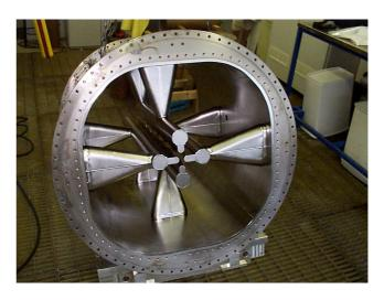
Figure 2 .SRFQ2 resonator at the final stage of rinsing, prior to installation into the test cryostat.
