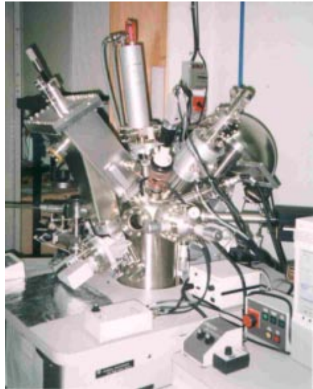
Figure 7, XPS Auger Surface Analysis System used for Surface investigation of the Niobium properties.
